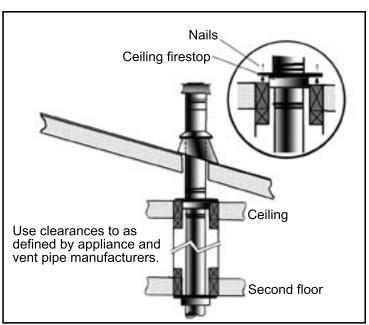
Figure 31: Multi-Story Vent Pipe Installation.
